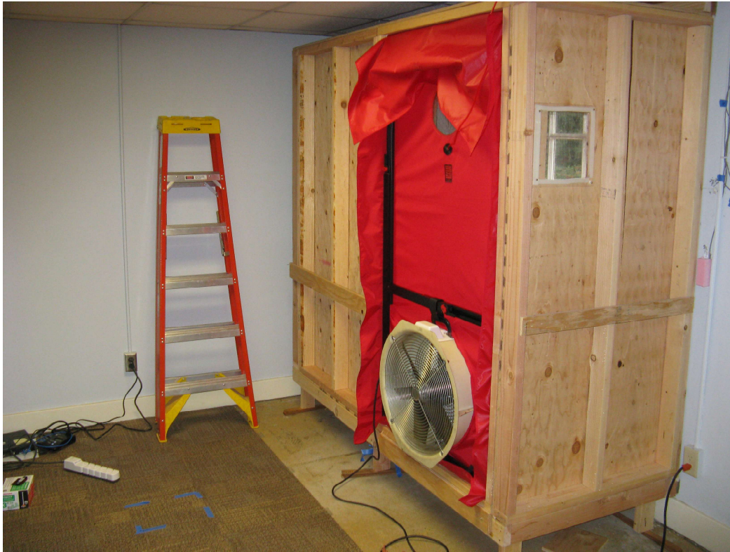
Figure 4, Blower Door Testing in Meter Chamber
